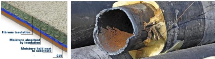
**Gambar 8.** ilustrasi *corrosion under insulation*.
